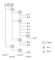
The VM9324 player will only recognize three folder levels and does not display folders containing only other folders. In the example above, the unit will display folders 3, 4, 6, and 8, but not 2 and 7 since they do not contain any tracks directly. Folder 5 is not recognized at all since it is at the fourth level.
